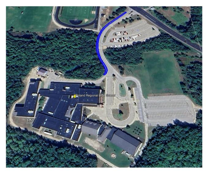
Blue = New asphalt curbing and sidewalk paving (+/- 1,379 ft x 6 ft. wide)
