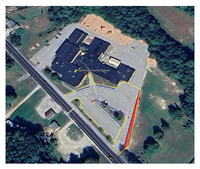
Yellow = Reclaim, shim, and overlay area (+/- 5,200 sq. yds.) Blue = New asphalt curbing and sidewalk paving (+/- 440 ft) Red = Fine grade and add new pavement (+/- 226 sq. yds.)
